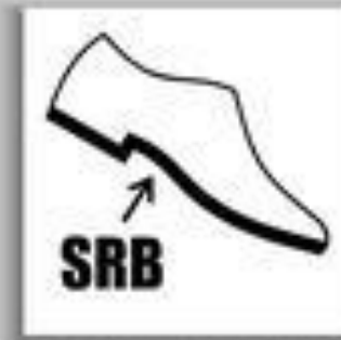
SLIP RESISTANCE ON STEEL FLOOR WITH GLYCERIN
